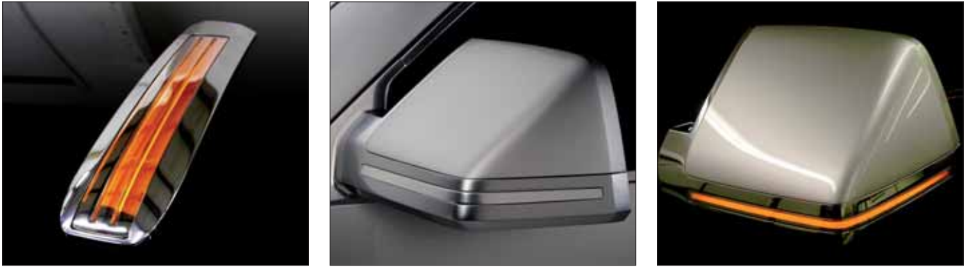
Figure 2. Stealth lighting using transparent chrome. Left: one of several chrome bezels placed on the outside front of the glass roof. The LED lighting is beneath the glass. Middle and right: wing mirrors with amber LED indicators.
