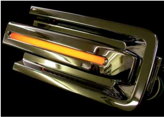
Figure 3. Door handles containing a custom-made LED light-guide are a hugely popular feature of the Ford Super Chief concept.
