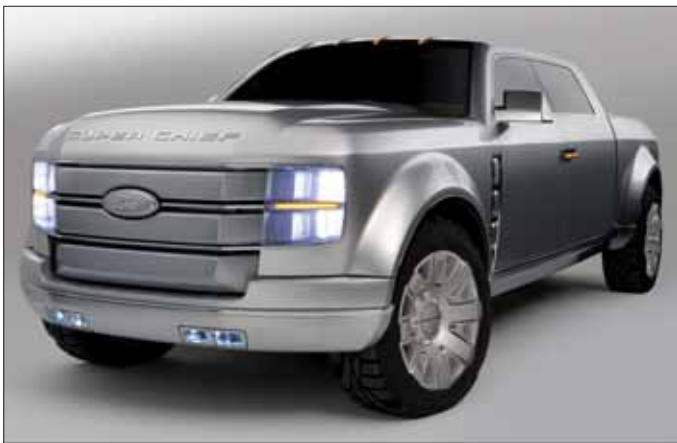
Figure 1. The front of the Ford Super Chief concept has white LED forward and fog lights, as well as amber “transparent chrome” running lights on the roof. The front indicator and door handle lights are made with LED light guides. The rear features horizontal light guides, as well as multiple LED brake light units on the roof.
